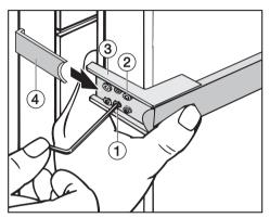
Loosely attach the handle to the opposite side of the door with the two front screws 2.
